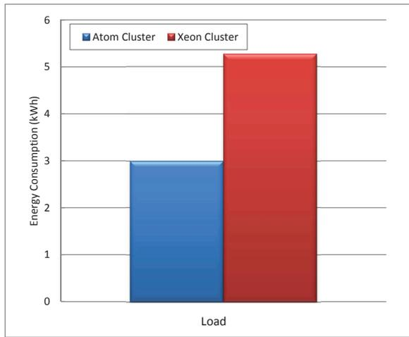
**Figure 3: Total energy consumption comparison between a 30-node Atom cluster and a 15-node Xeon cluster**
